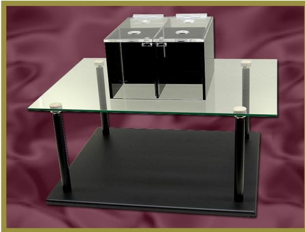
\*Due to the fact that glass acts as a heat sink\*; IITC developed the only commercially available heated glass. Warming the glass eliminates the heat sink problem, thus animals are placed onto the slightly warmed glass. Builtin temperature controller in the heated base version keeps glass at a constant temperature between 30-40 deg. C. which can be adjusted by user as needed.
